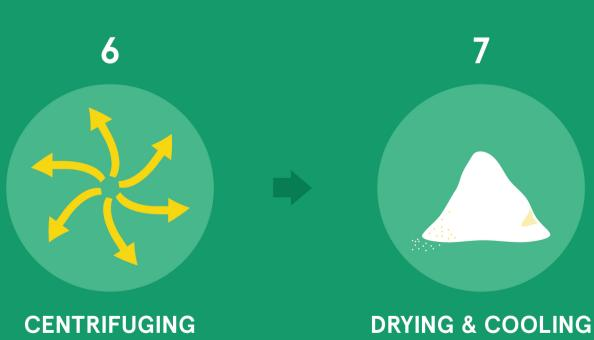
Centrifuge **separates**the white sugar crystals from
